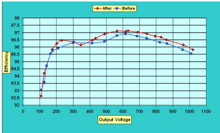
**Fig.11** Efficiency as a function of output voltage for the CPE 5:1 wide ranging power supply. The red data points were obtained after optimization of the 3-phase resonance circuits. All data shown were obtained at a constant output power level of 1 kW.
